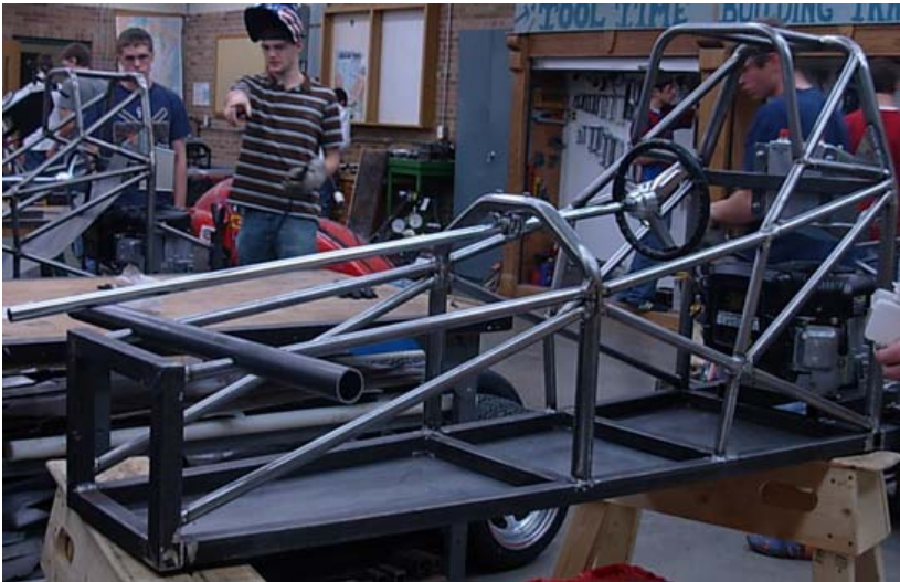
Our chassis with the engine, fuel cell, and our steering wheel installed
